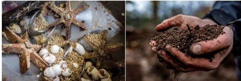
ABB safety products ensure machine safety. It is absolutely impossible to start the machine unless the safety sensor has confirmed that all doors are closed. The temperature can reach 63°C inside the machine, as microorganisms help break down old bread, potatoes and egg shell.
