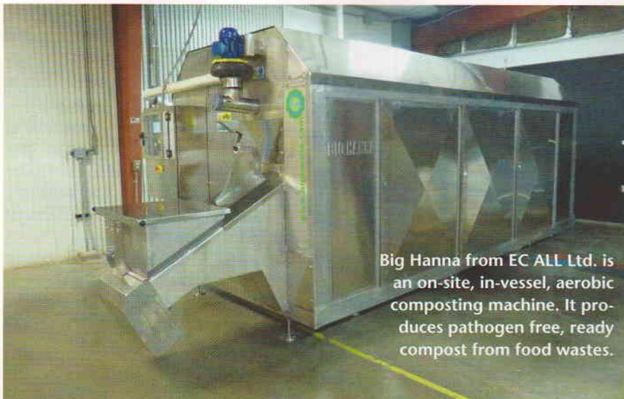
Big Hanna from EC ALL Ltd. is an on-site, in-vessel, aerobic composting machine. It produces pathogen free, ready compost from food wastes.
